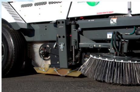
**DUST SUPPRESSION SYSTEM** • **Global M4** includes **250-Gallon Water Tank Capacity** combined with Two(2) Diaphragm Water pumps and Two(2) Modes (LOW/HIGH) provide versatility and superb dust control.
