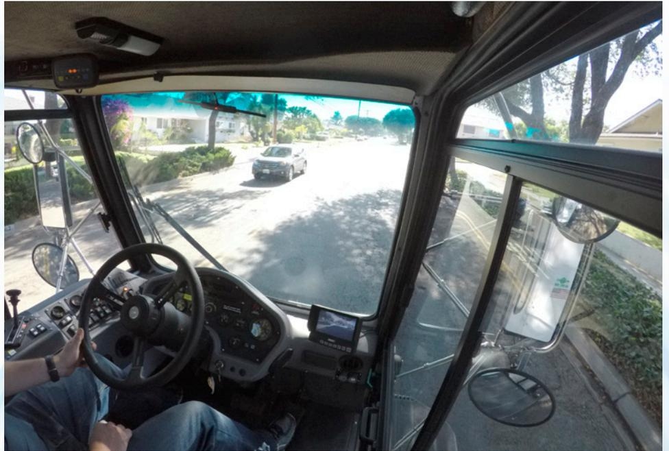
The inherent design of the **Global M4** makes it the logical choice among heavy-duty mechanical sweepers. With the center mounted/cab forward layout the operator has unsurpassed visibility of the road surface as well as pedestrians and surrounding traffic. The large hopper capacity equals more lane miles swept between dump cycles and the **18.5-foot turning radius** makes the **Global M4** highly efficient and comfortable.
