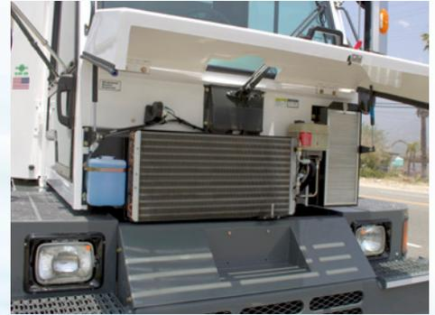
**ACCESS IT ALL** The *Global M4* features many maintenance-friendly attributes, such as a rear swing-out radiator, easy access front mounted AC condenser, brake and windshield washer fluid reservoirs, and cab fresh air filter.
