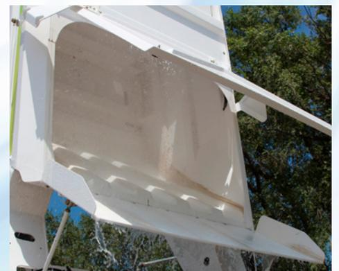
**Global M4** includes a **5.6 cu/yd hopper capacity** compared to 4.5 cu/yd for competitive machines resulting in more curb miles swept between dump cycles. With near Full Useable Capacity, 12,000 Lift Capacity, and the Optional Elevator and Hopper Wash Out System, **Global M4** is **Affordable, Reliable and Innovative**.
