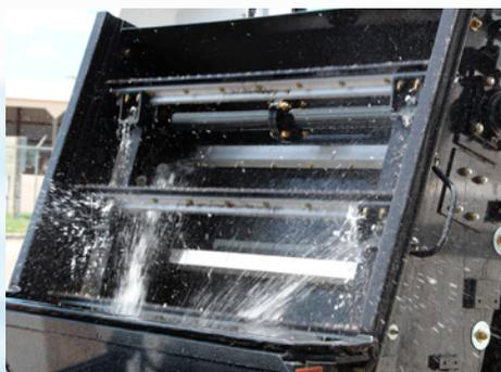
**HEAVY SWEEP PACKAGE** Elevator Type: Standard 11 Flight squeegee with replaceable corded rubber tips; Continuous molded rubber belts combined with standard Heavy Sweep Package make **Global M4** the logical choice for sweeping heavy debris such as road millings, sand and gravel up to **3-Tons per-Minute**. That is one ton of sand every 20 seconds! Standard leaf gate system assists in picking up large debris, bottles, large branches and leaves.
