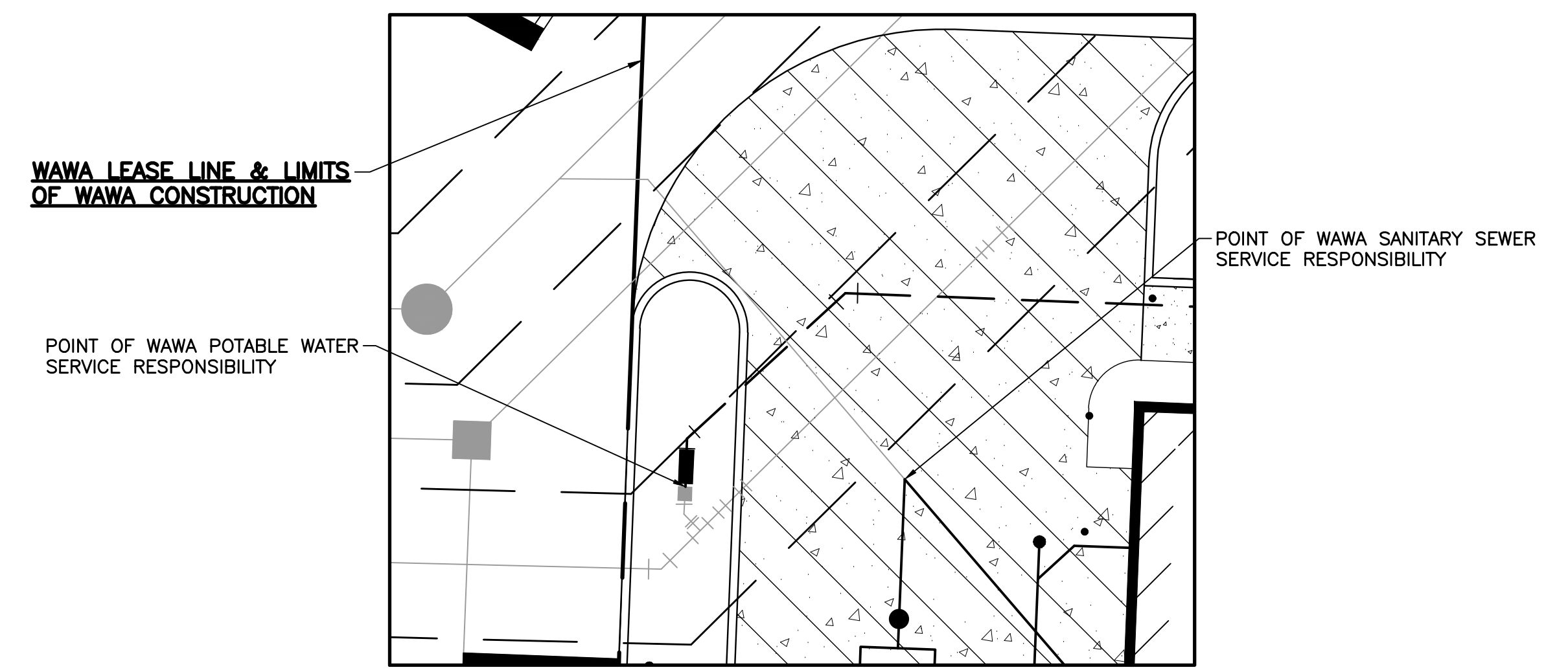
DETAIL "A" WATER & SANITARY SEWER CONNECTION SCALE 1"=10'
